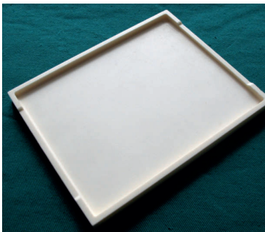
Fig. 6 Stackable box setter system in mullite E to fire MLCC. ZrO 2 coating will be applied onto the setter to prevent contact reactions
