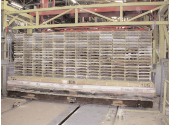
Fig. 6a Industrial test of Aptalite. Aptalite cassette (white) irregularly placed onto a kiln car.
