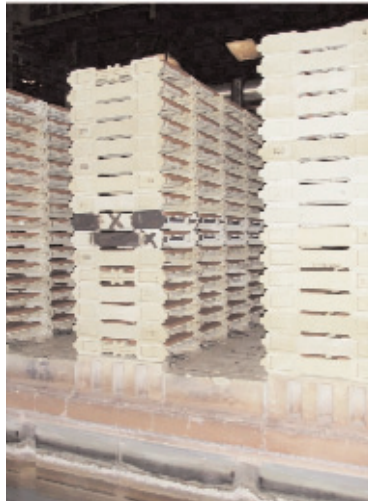
Fig. 6b Industrial test of Aptalite: marked Aptalite among standard IKF-cassettes on a kiln car.
